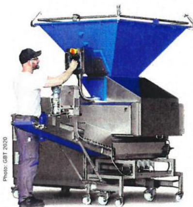
The Olympia works with a curve control with adjustable moulding pressure, weight-dependent press stroke and adjustable speed for cycles and belts.
