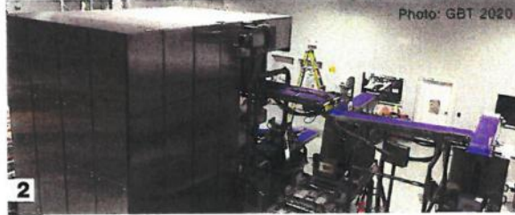
1 This bread line comprises the Olympia H2, the Konus V5000 conical rounder, an intermediate proofer with pallet infeed, 12 rows and 80 dough carriers, as well as the LR6W4B2 moulder. 2 The intermediate proofer is completely covered with clip-on V2A panels. It is also electrically protected and has large sliding viewing windows made of Makrolon. 3 This shows the Olympia's main piston and cutter. 4 The metering piston inserts can be used as required. Pump piston and cutter are mechanically driven by a cam disc.
