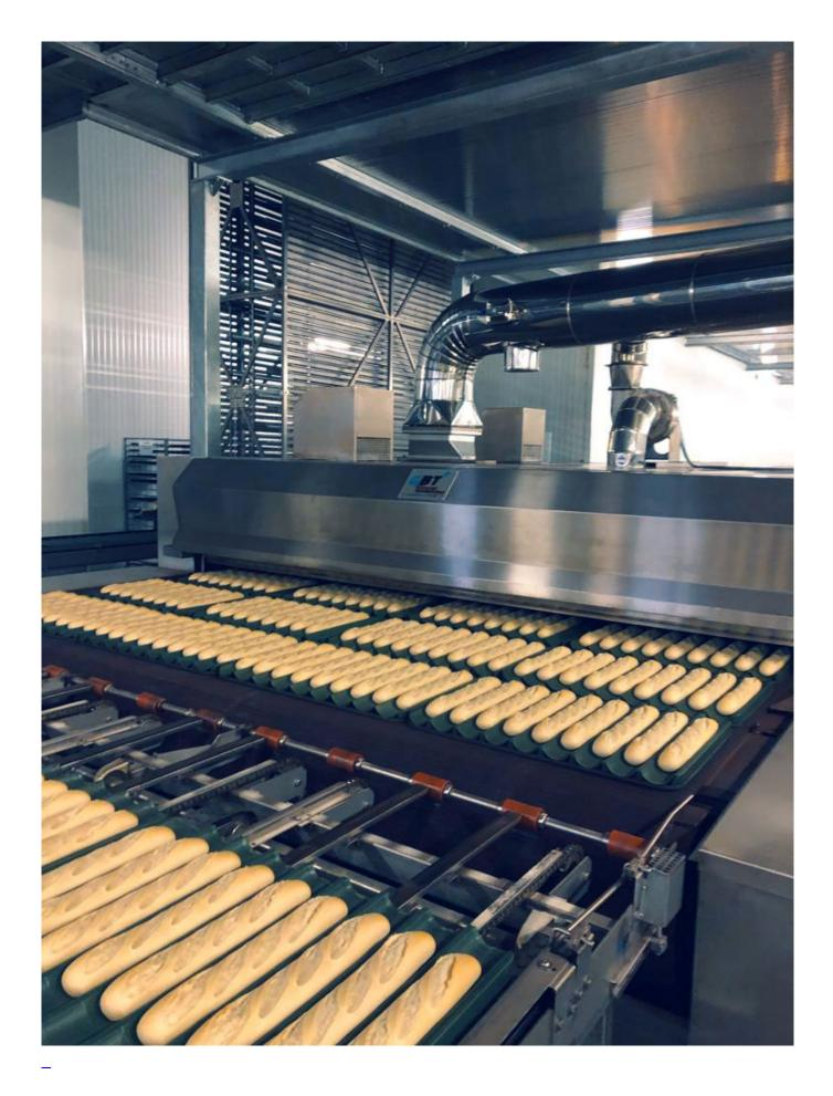
This industrial bread baking plant situated near Barcelona reaches an output of up to 5,000 pc. par-baked baguettes thanks to GBT's oven Mistral. Far beyond: The energy optimized modular conveyor oven saves up to 30 % of energy in comparison with a conventional cyclothermic oven. This is possible due to the specially developed use of the flue gases energy. Typically GBT: maximizing output, reducing energy consumption.
