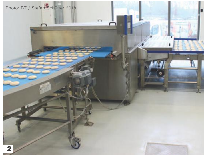
1 The line's input interface for the new modules from GBT and the oven from Heuft can be found at the baking chamber's exit. 2 The oven is currently being supplied by a six-line baking system. However, the transfer system has been designed to operate as an eight-line system.
