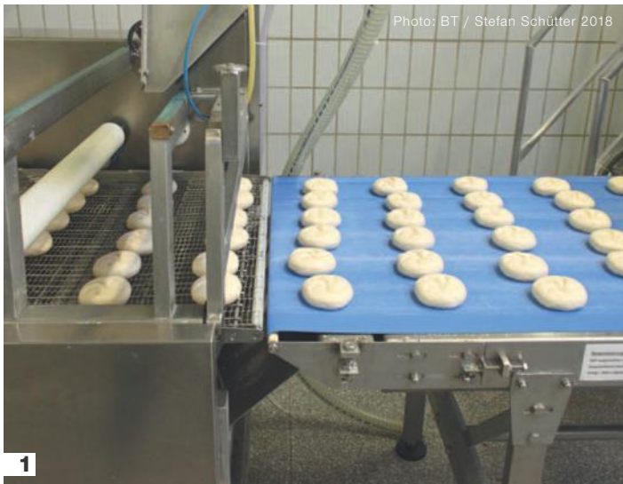
1 The line's input interface for the new modules from GBT and the oven from Heuft can be found at the baking chamber's exit. 2 The oven is currently being supplied by a six-line baking system. However, the transfer system has been designed to operate as an eight-line system.
